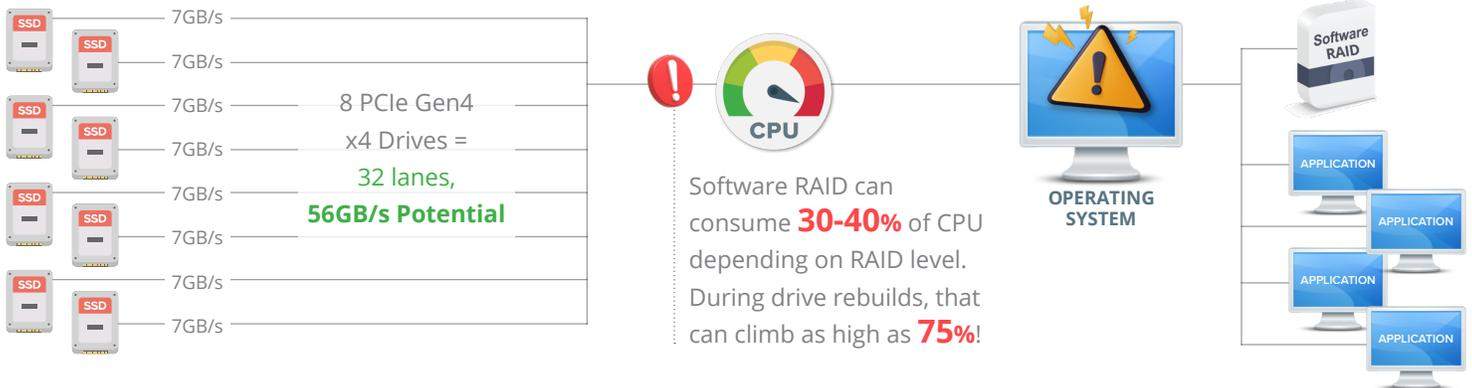
...but SupremeRAID™ GPU-based RAID eliminates the RAID bottleneck without taxing the CPU, and achieves the full potential of your SSD performance.
