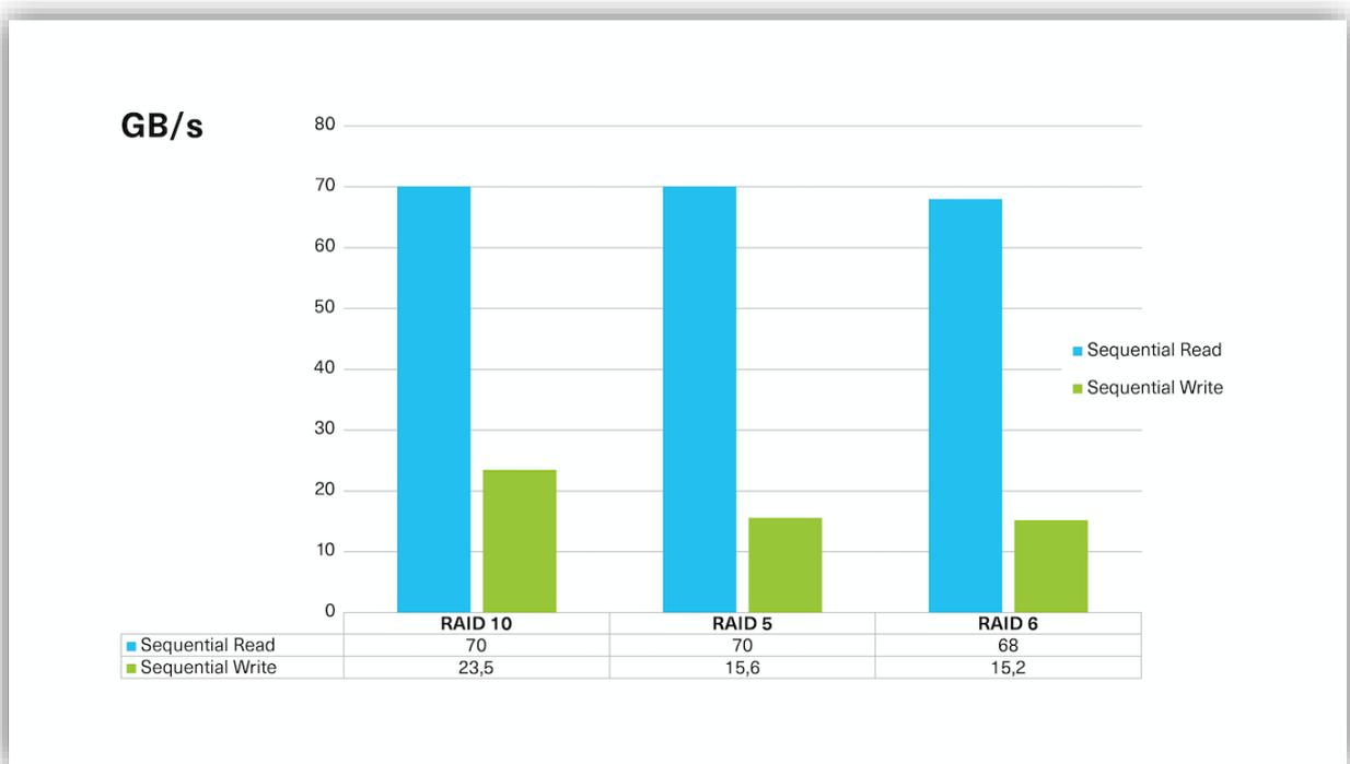
Figure 4: RAID performance, sequential reads and writes
