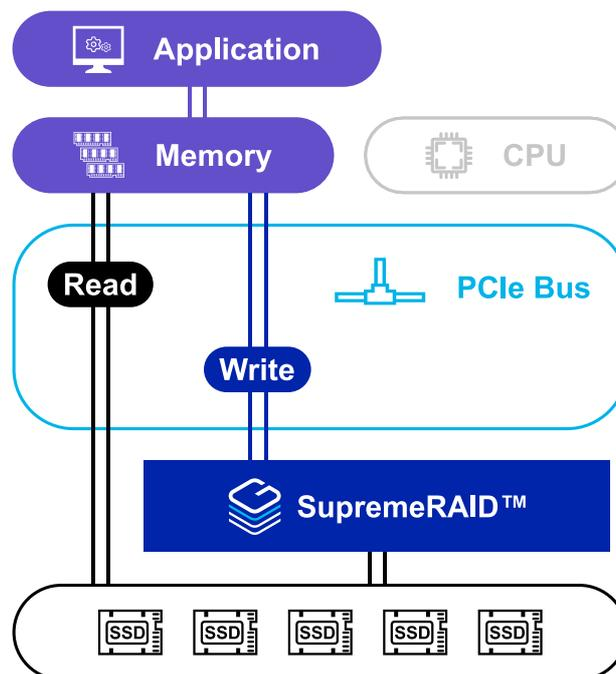
Figure 1: SupremeRAID™ by Graid Technology enables high performance with low CPU load.
